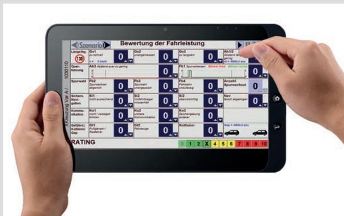
**73** The tablet application S. A. F. E. for a semi-automatic registration and classification of driving errors developed by the WIVW ([www.wivw.de](http://www.wivw.de))
