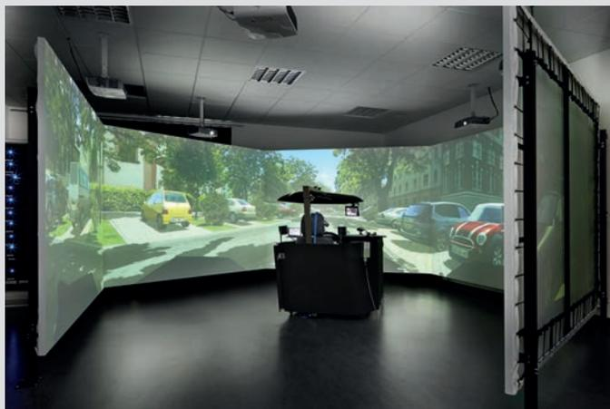
Figure 1: Fixed base driving simulator of the WIVW
